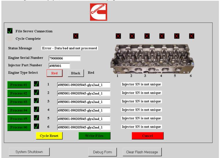
This screen directs the user to scan 6 fuel injectors and then validates the data before sending it to the customer's data system.
