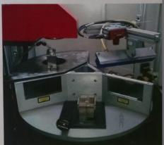
PW gets part type from plc. Checks correct part type by read RF id tag on pallet. Nests are unique to part type. Sends file to laser; triggers laser; mark complete; rotates turntable; fires camera to verify quality; sends results back to PW
