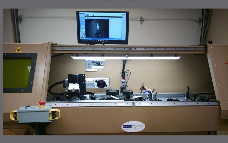
After the parts are marked they are checked for good mark quality and decode content. Each part is uniquely identified and the data is associated with the part is logged to Plantwatch. Latter this data will be used to verify that the mark quality was good before any work is done with the part.
